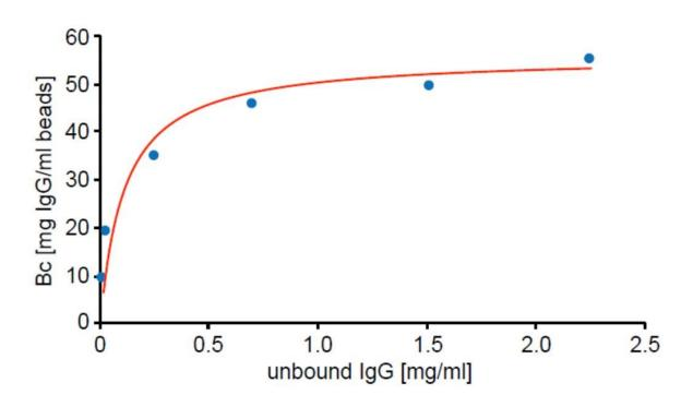
Binding capacity assay with a humanized mAb IgG1 on the magnetic protein A agarose beads, MAGicBeads PrtA. Static binding capacity from adsorption equilibrium experiments fitted with Langmuir isotherm.
